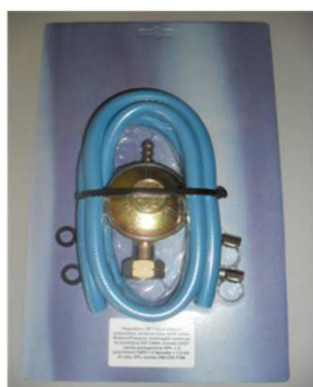
SKINPACK KIT WITH 1 Kg./h REGULATOR EN 16129 NORM - SEAL - 2 CLIPS - 1,2 mt. GAS PIPE UNI 7140 NORM
