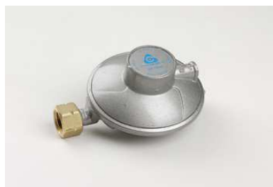
HORIZONTAL LOW PRESSURE 3 KG/H LPG REGULATOR FIXED ADJUSTMENT FOR DOMESTIC USE EN 16129 NORM
